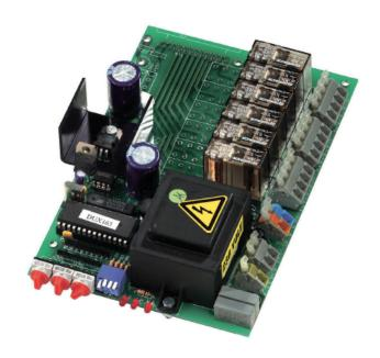
MA demultiplexers receive DMX512 signals and convert them. For reasons of data integrity, any tapping of DMX signals is protected against over-voltage on MA devices.
