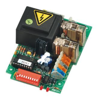
MA demultiplexers receive DMX512 signals and convert them. For reasons of data integrity, any tapping of DMX signals is protected against over-voltage on MA devices.
