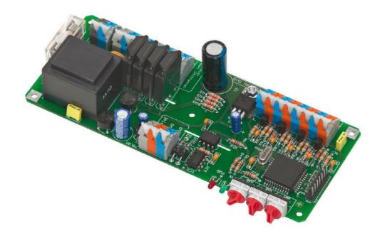
MA demultiplexers receive DMX512 signals and convert them. For reasons of data integrity, any tapping of DMX signals is protected against over-voltage on MA devices.
