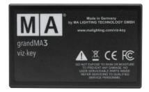
The grandMA3 viz-key is the unique solution for a stable and safe connectivity between third-party visualization tools and grandMA3 lighting control systems. Simply connect the grandMA3 viz-key with the visualization computer and it will enable all necessary parameters for visualization. The external visualizer will be recognized as a MA-Net3 device in the network for a direct connection to your grandMA3 session.
