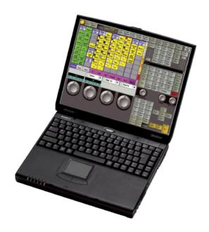
The grandMA onPC software is not only a PC emulation of an entire grandMA console for the editing and processing of show data, but in cooperation with the MA NSP it can also control up to 4,096 parameters (512/1,024 parameters with the MA 2Port Node onPC/Pcpro).
